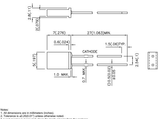
3. Lead spacing is measured where the leads emerge from the package.
